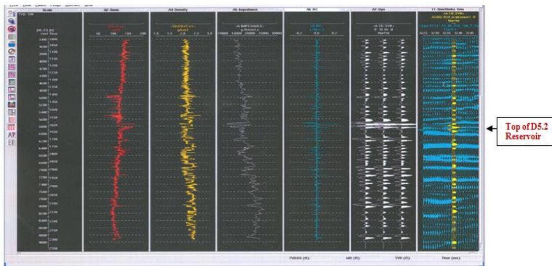
**Figure 6:** Agbada Field: Well-to-Seismic Tie for Well "X" showing the top of D5.2 Reservoir
